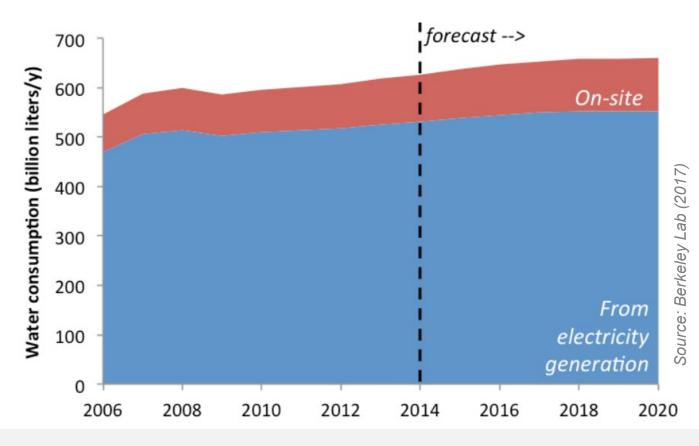
Figure 25. Direct vs. Indirect U.S. Data Center Water Consumption
